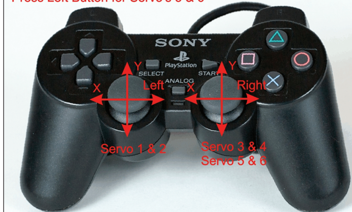
FIGURE 12. Servomotors mapped to PlayStation controller.
