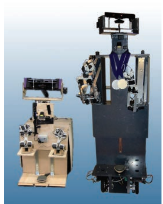
FIGURE 2. The first prototype (left) beside the new and improved PVC PR2Lite (right).
