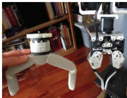
FIGURE 10. A Velo gripper (left), courtesy of Willow Garage next to our current gripper (right). The Velo is already larger than the current gripper, and it will be even bigger and heavier with servos.
