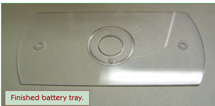
Use a template to cut out the battery tray.
