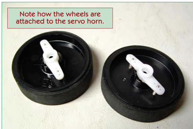
The finished motor/wheel assembly.
