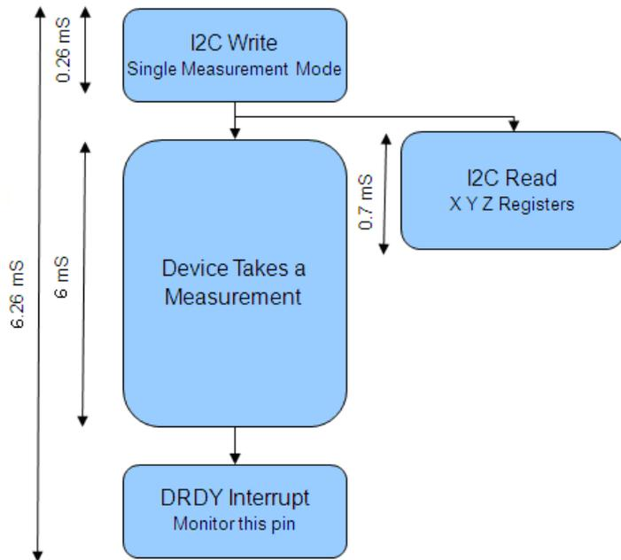
\* Monitoring of the DRDY Interrupt pin is only required if maximum output rate is desired.
