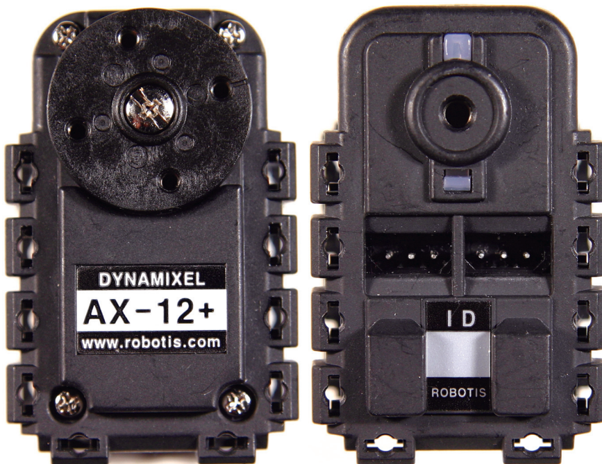
PHOTO 1. The daisy-chained one-wire RS-232 link I am referring to is actually a DATA line and a GROUND line. The AX-12+ also distributes power on a third daisy-chained line.
