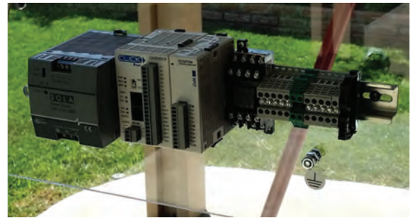
Figure 11. From left to right, 24 VDC power, PLC, TC module, relays, and DIN rail terminal blocks.
