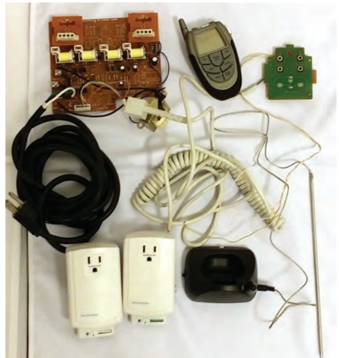
Figure 4. Rev 1 electronics, bed controller, Insteon discrete and relay modules, and thermometer.
