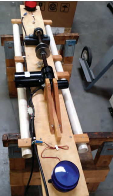
Figure 8. Rev 2 winch bearing and spool guides.
