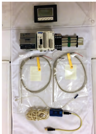
Figure 13. Rev 2 electronics. Top to bottom, display, PLC system, thermocouples, Hall-effect sensor, and programming cable.
