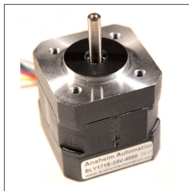
Photo 1. This BLDC motor comes ready to work with drive circuitry that employs the use of its built-in Hall effect sensors. These sensors are ignored when the motor is spun using sensorless BLDC motor drive techniques.
