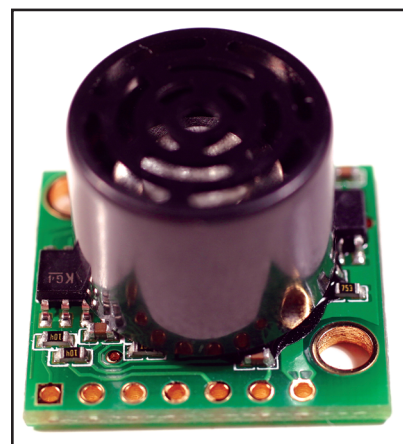
PHOTO 1. The LV-MaxSonar-EZ0 you see here is a combination of the MaxBotix MaxSonar-UT ultrasonic transducer and the proprietary circuitry you see in Schematic 1. Another reason for not getting too deep with the inner workings of the EZ0 is that there is no technical information available from MaxBotix for the ultrasonic transducer.
