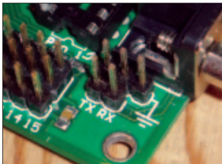
Figure 7. Close-up view of the TX and RX pins on the SSC-32.
