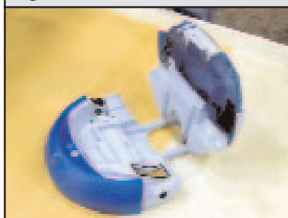
Figure 5. The inside of the Scooba.
